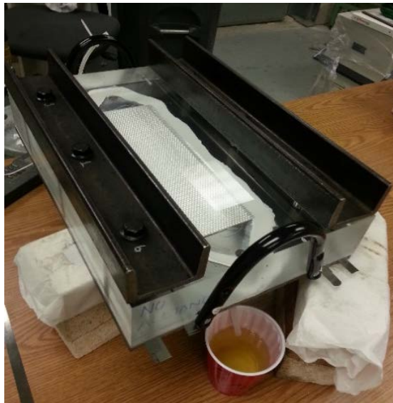
Figure 3-5: Second Tool with 3” Thick Acrylic
